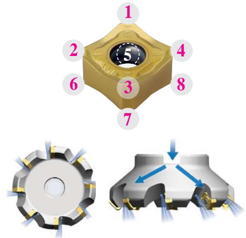
► Through coolant system for decreasing cutting heat and good chip evacuation
